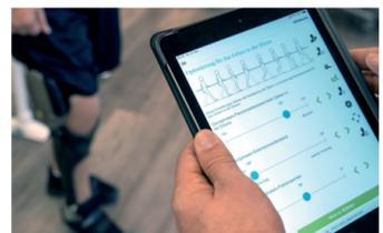
Abb. 6: Gangphasencheck via App & Tablet-Computer
